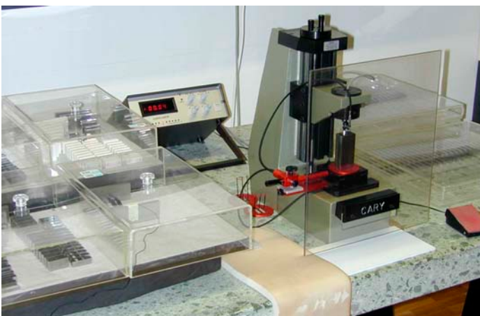
Figure 2. Gauge block comparator at METAS.
