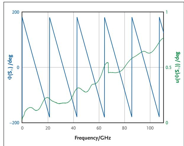
6: Phase of  $S_{11}$  of one of the 1.0 mm offset short standards in blue, bounded by the associated standard uncertainty interval in green.
