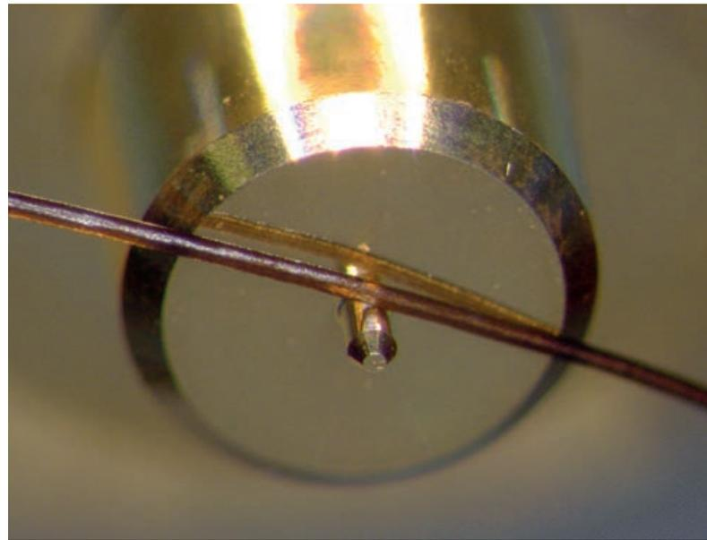
1: 1.0 mm male flush short, consisting of a short plane and a male pin, in comparison with a human hair.
