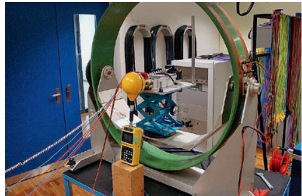
5: Magnetic induction influence up to 2 mT, compared to 0.5 mT in traditional meters.
