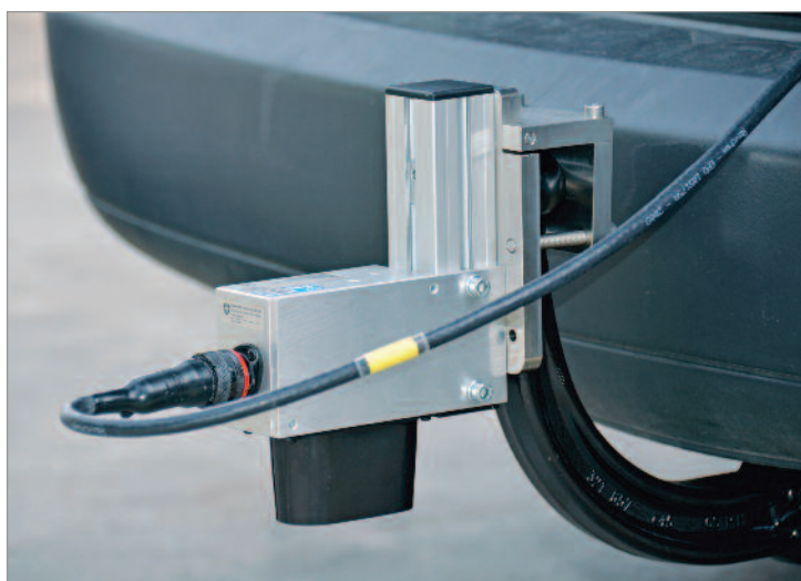
Figure 3 Optical correlator mounted on the METAS vehicle
