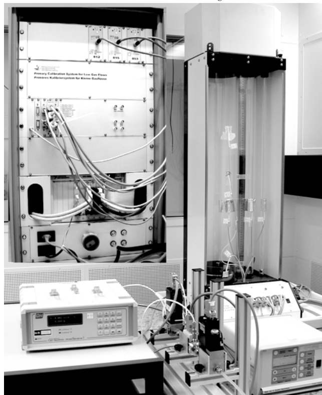
Figure 1: Picture of primary volumeter for low gas flows at METAS with separate electronics
