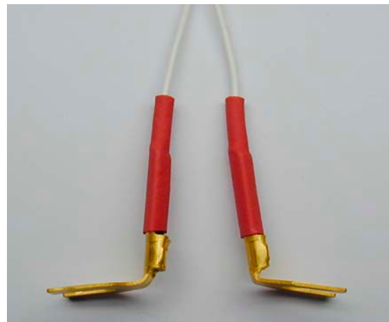
Picture 2: Inward and outward bending of the lug to make connections easier.
