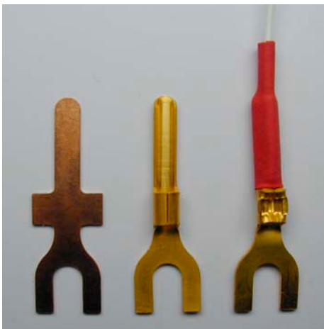
Picture 1: from the left: raw copper lug, finished gold plated lug, lug mounted on a cable
