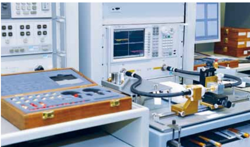
1 A vector network analyser is used to measure S-parameters, which are fundamental quantities in RF & MW metrology.
