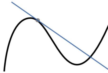
Figure: The graph of a function, drawn in black, and a tangent line to that function, drawn in blue. The slope of the tangent line is equal to the derivative of the function at the marked point.
